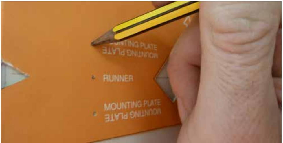
9. Mark the centre positions for the drawer runners from the inside of the carcass, using the supplied tape measure and the heights shown in the chosen “Carcass illustration”, accuracy here will ensure smooth running of the drawers.
