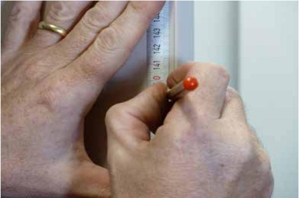
5. Extend the marks horizontally using a set / combination square, placed against the carcass front edge for each hinge mounting plate position on the carcass.
